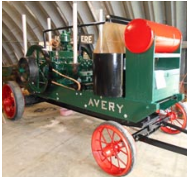
MAPA's 50HP Avery stationary engine, which was totally restored by members of the "A Team", in celebration of our 40th Anniversary in 2013.
