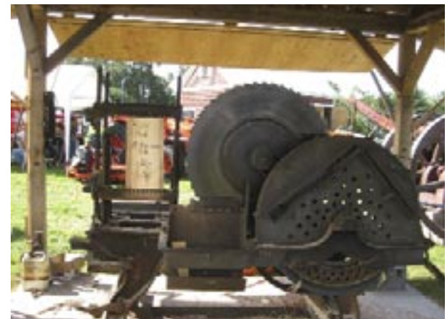
A Lane shingle mill ready for its' next demo at the Raitt Farm Homestead Tractor and Engine Show in Eliot, ME.
