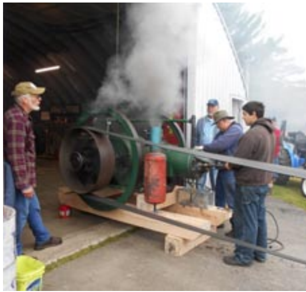
MAPA's 20HP Fairbanks Morse Style Y Semi Diesel, being fired up after not being run in many years, in honor of our 40th Anniversary.
